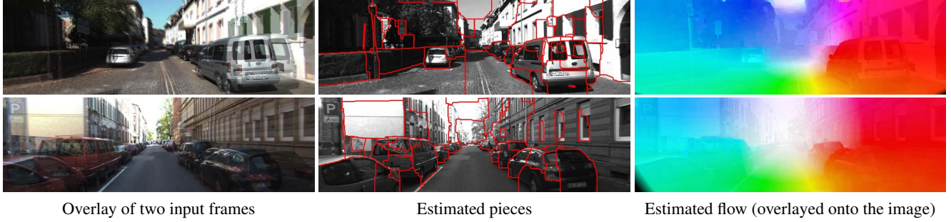
Figure 4: Example results of our method on KITTI benchmark. Note that in the example of the first row, motions of small objects such the road lamp and sign are successfully estimated (flow color scheme of the benchmark is used).
