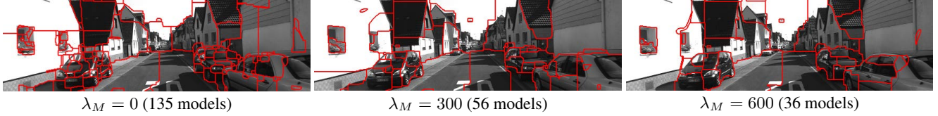
Figure 3: Effects of different MDL weights. Larger MDL weight leads to less homography models and larger pieces. We found that usually around 40~80 homography models are adequate for flow estimation on KITTI benchmark.
